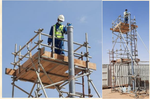
Level Transmitters Testing Radar / Ultrasonic
